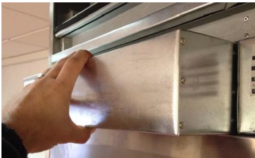
Sliding Back the Stage 3 Filter Panel
