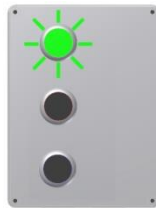
Flashing Green Machine Stopping
