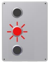
Flashing Red WARNING! Machine Stopped
