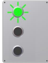
Flashing Green Machine Stopping
