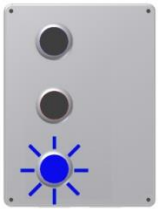
Flashing Blue Machine in Cleaning Mode – Bin Full
